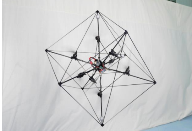
Fig. 6 Omni-directional aerial vehicle developed at ETH [6].
